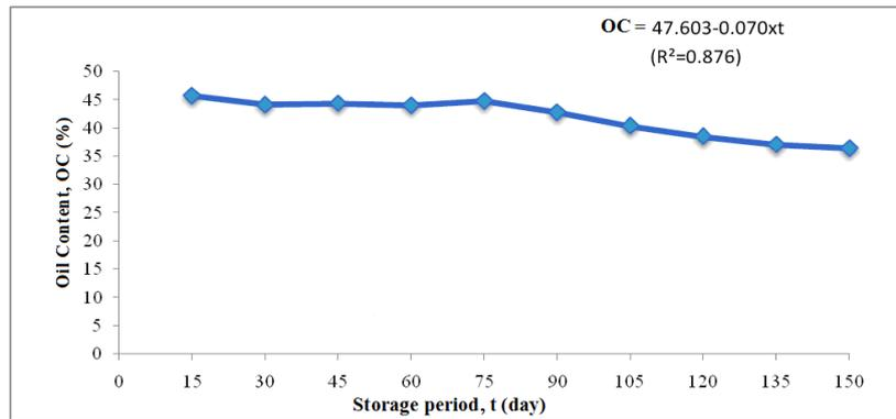
Fig.6.The effect of storage period on the oil content (OC)
