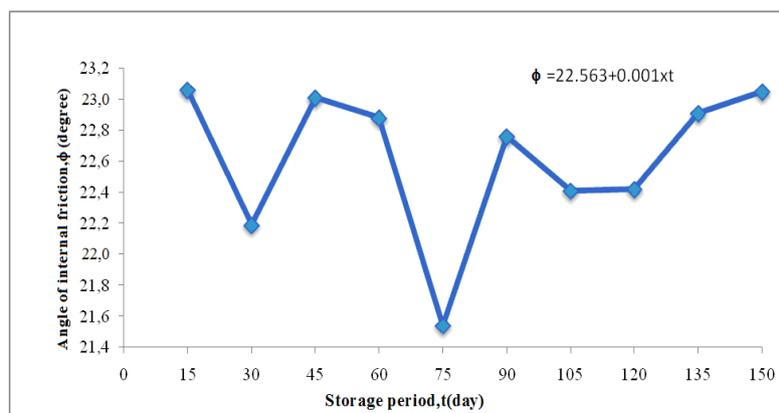
Fig.4. The effect of storage period on angle of internal friction
