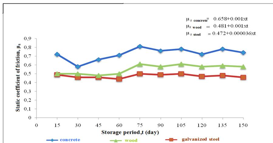
Fig.5. The effect of storage period on static coefficient of friction
