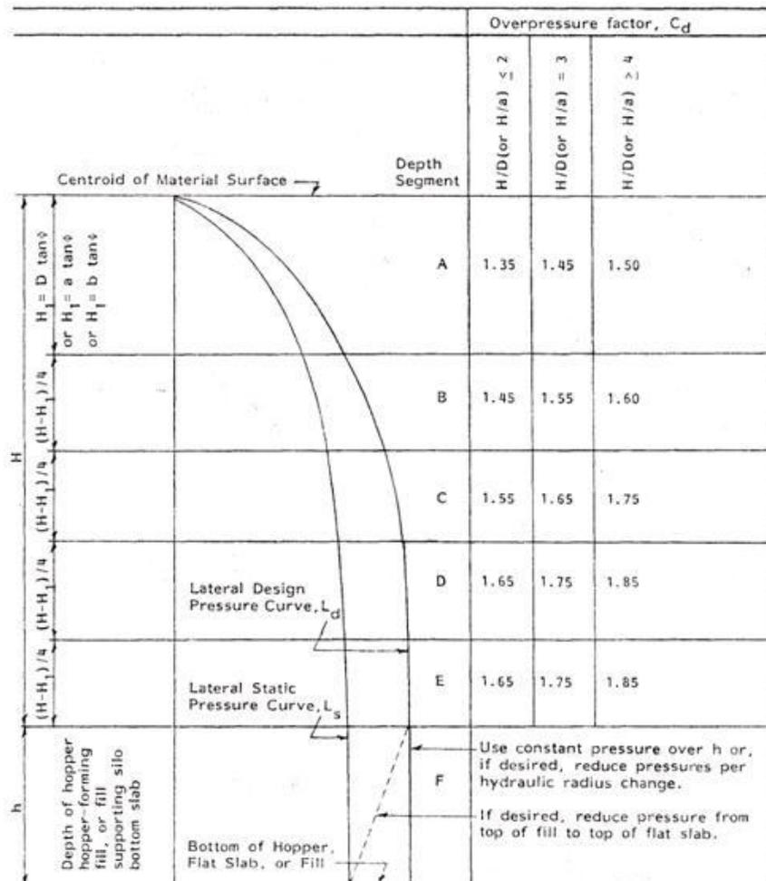
Figure 3. Minimum over-pressure factors,  $C_d$ , for deep bins (MWPS, 1983)
