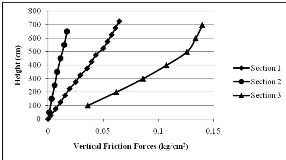
Figure 6. Change in vertical frictional forces
