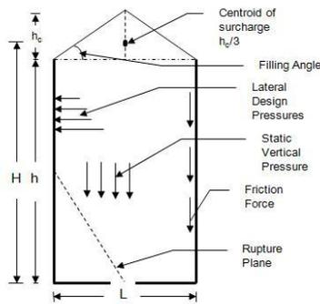
Figure 2. Loads acting in a silo
