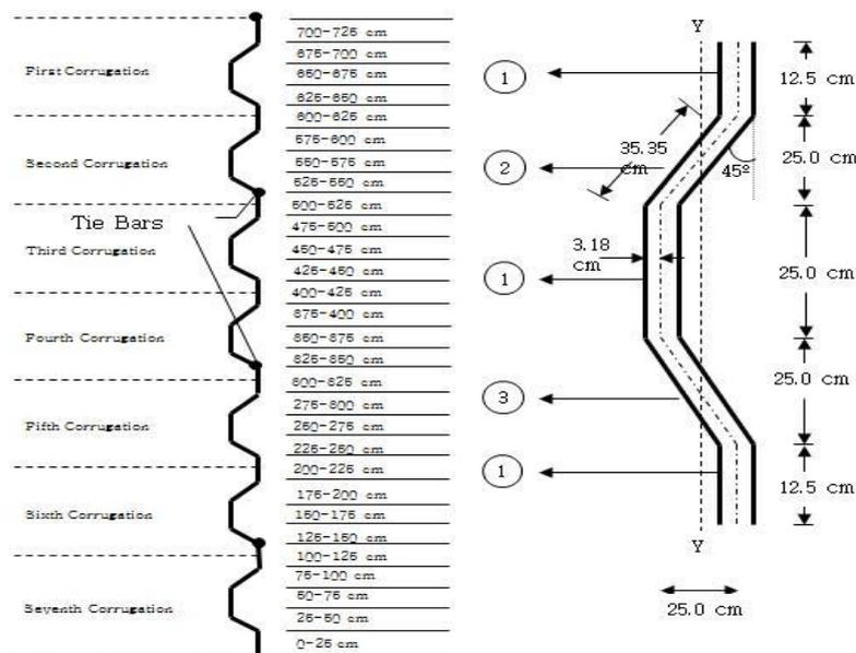
Figure 4. Corrugation numbers, elevations, dimensions and sections
