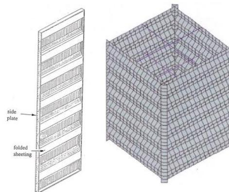
Figure 1. Pre-fabricated wall panel and bin configuration
