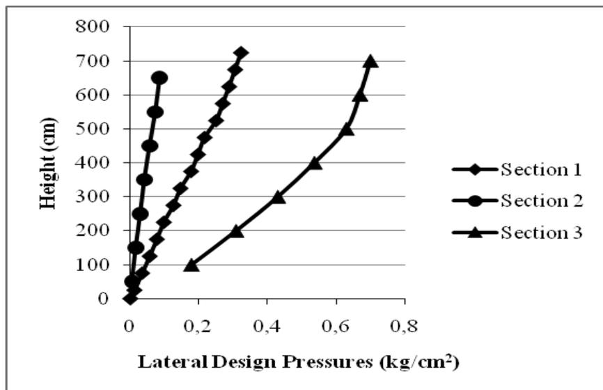
Figure 5. Change in lateral design pressures
