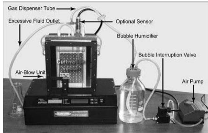
**Figure 1.** FMT-150 photobioreactor
