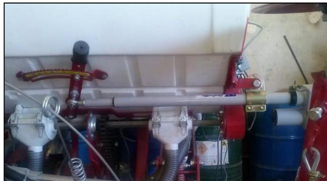
**Figure 1.** Flow rate control mechanism
