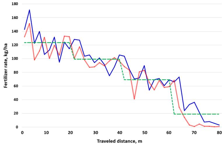
**Figure 6.** Variation in fertilizer rate with traveled distance at decreasing transition order ( — collected from right hopper and — collected from left hopper represents observed data and - - - dashed line represent mean value for each fertilizer rate)
