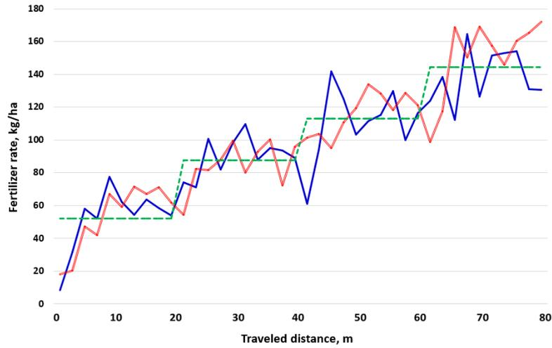
**Figure 5.** Variation in fertilizer rate with traveled distance at increasing transition order ( — collected from right hopper and — collected from left hopper represents observed data and - - - dashed line represent mean value for each fertilizer rate).
