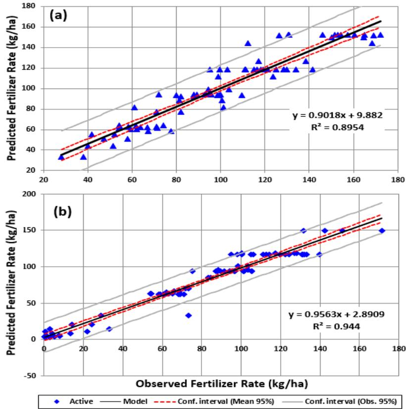
**Figure 7.** Relation between predicted and observed fertilizer rates during test procedure for increasing transition order (a) and decreasing transition order (b). The total number (n) of samples in each plot is 80
