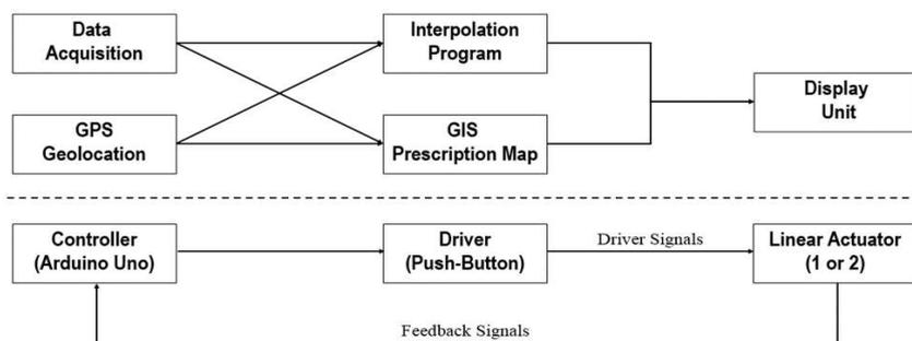
**Figure 2.** Block design of manual type variable rate fertilizer
