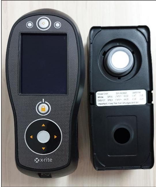
**Figure 2.** X-Rite Ci60 portable spectrophotometer
