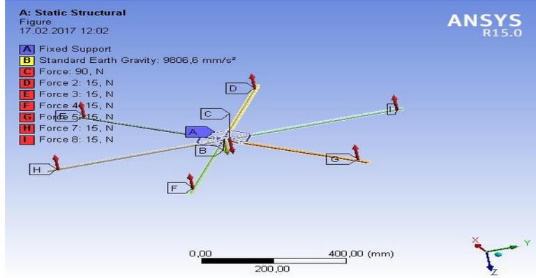
**Figure 2.** Schematic view of the force values used for the analysis.
