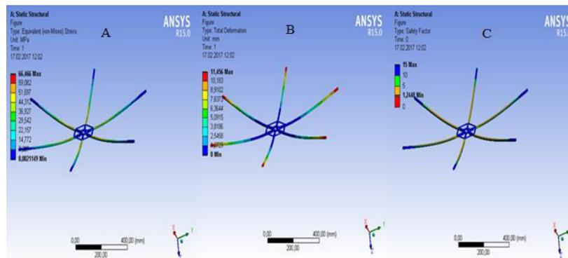
**Figure 7.** The values in the analysis results (A-Total stress, B-Total deformation, C- Safety factor).
