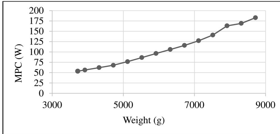
**Figure 9.** Weight-dependent motor power consumption.
