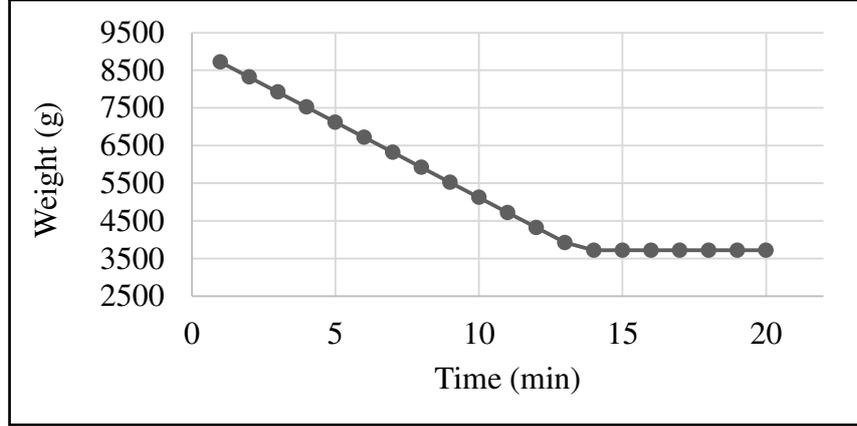
**Figure 8.** Time-dependent weight reduction during the UAV operation.
